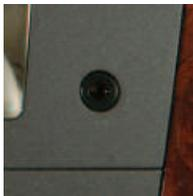
There is an auxiliary input jack on the lower right of the audio system faceplate. You can connect an external audio
