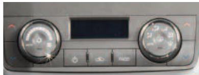
The dual-zone climate control system can be operated manually or can be set to automatically adjust to the individual settings of the driver and front seat passenger.
