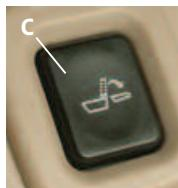
Press and hold either folding button to fold or unfold the seat.
