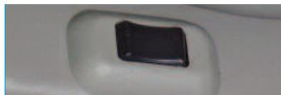
The power lumbar switch is located beneath the power seat switch controls. Hold the control forward or rearward to increase or decrease support.
