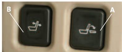
Two buttons are located on the right-side panel behind the second-row seat. One button (A) folds and raises the seat and another button (B) changes the seatback angle.
