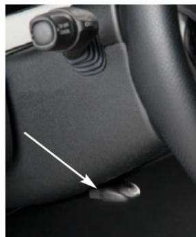
To tilt and telescope the position of the steering wheel:
