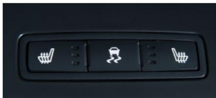
The heated seat buttons are located at the front of the center console.
