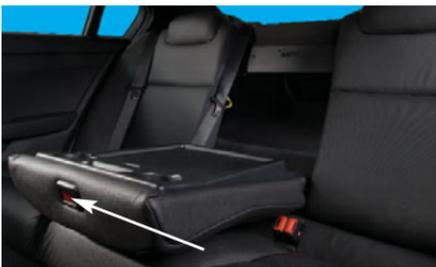
The rear seat has a center pass-through section that may be folded forward to gain access to the trunk or for carrying long loads. The back of the pass-through also has two cupholders.
