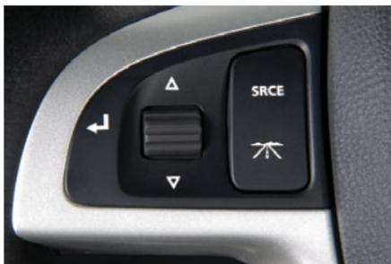
The following audio controls are located on the steering wheel:
