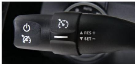
Cruise control is operated by using the multifunction lever on the left side of the steering column.
