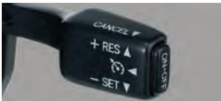
The cruise control lever is located on the lower-right side of the steering wheel.
