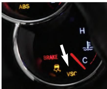
StabiliTrak is a Vehicle Stability Control (VSC) system that uses an advanced computer to assist your vehicle with directional control during difficult driving situations.
