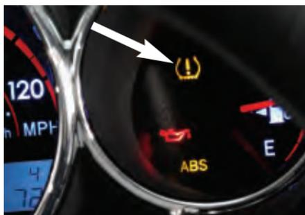
The Tire Pressure Monitor alerts you when a significant reduction in pressure occurs in one or more of your vehicle's tires by illuminating the (⚠) (Low Tire Pressure) warning light on the instrument panel. The low tire pressure warning light will remain on until you correct the tire pressure.
