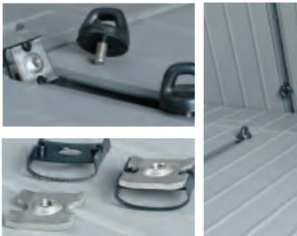
At vehicle delivery, cargo tie-downs and a corresponding installation diagram were provided under the rear cargo floor panel.
