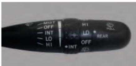
The lever on the upper-right side of the steering column controls the wipers and washers.
